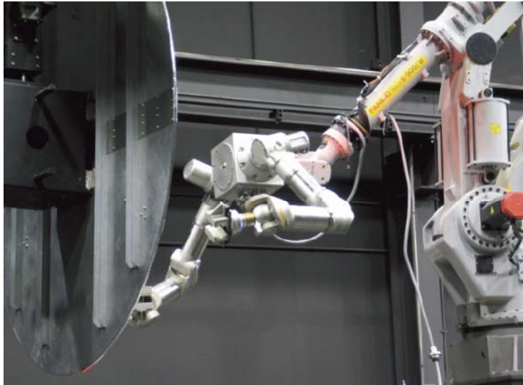
Ranger 8 DOF human-scale grappling arms. Ref: D. L. Akin, "Robotic and EVA/Robotic Servicing: Past Experiences, Future Promise," presented at the International Workshop on On-Orbit Satellite Servicing, Hosted by NASA Goddard Space Flight Center, Adelphi, MD, March 24-26, 2010, http://servicingstudy.gsfc.nasa.gov/ .
