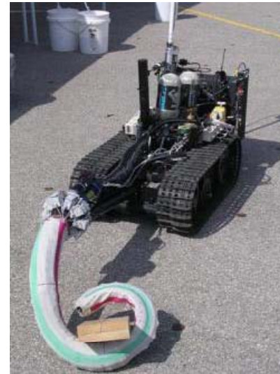
OctArm tentacle manipulators. Ref: D. Trivedi, C. D. Rahn, W. M. Kier and I. D. Walker, "Soft robotics: Biological inspiration, state of the art, and future research," Applied Bionics and Biomechanics , vol. 3, no. 5, pp. 99-117, September 2008.
